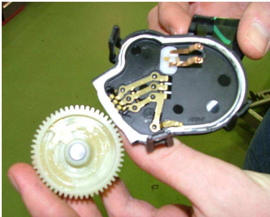
Replace it by the new engine wheel (*ref 2*) and the new cover (*ref 1*). Don't hesitate to apply some silicone all around the cover to seal it.
